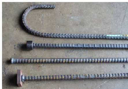
Fig. 3 Different headed bars and hooks bars
